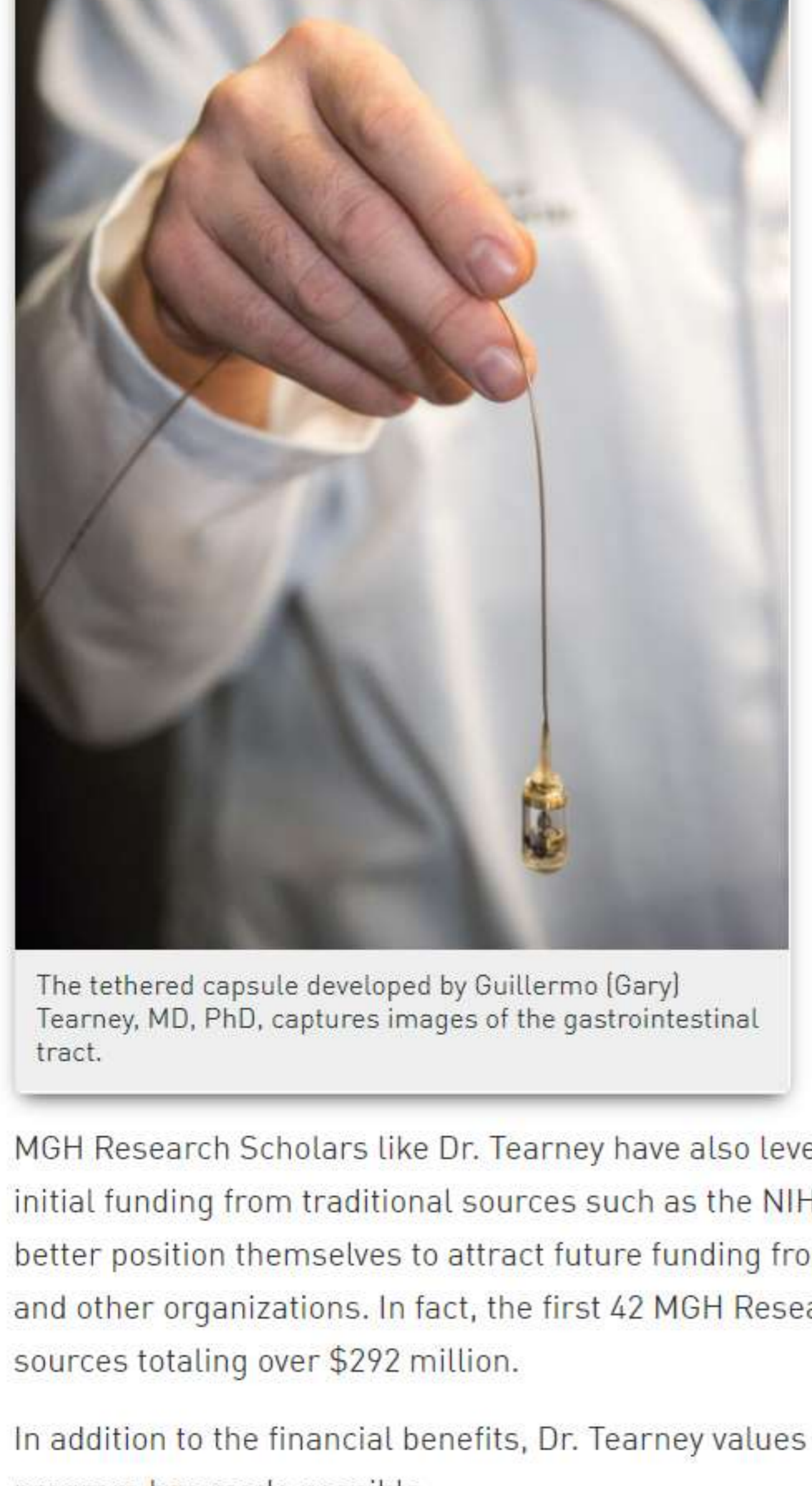
The tethered capsule developed by Guillermo (Gary) Tearney, MD, PhD, captures images of the gastrointestinal tract.
